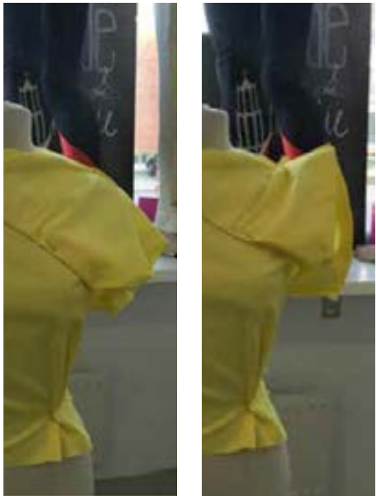
Figure 1. Sleeve activated by servomotors, Eindhoven 2018.
